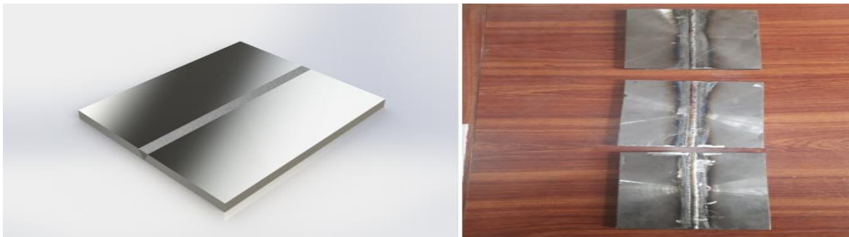
Figure 2. SMAW Welded AISI 316L ASS Plates Using Three Different Filler Materials
