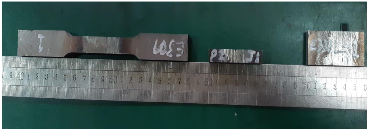
Figure 5. Physical Dimensions of Tensile, Impact and Hardness Specimens
