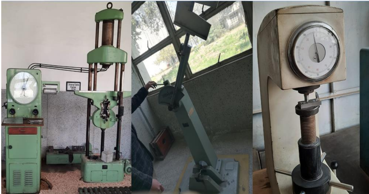
Figure 6. Tensile, Impact and Hardness Testing of Specimens
