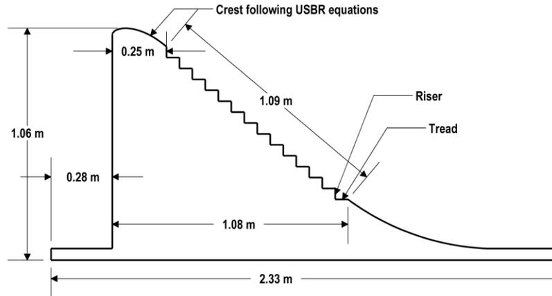
**Fig.4** Step configuration for C0 stepped spillway model
