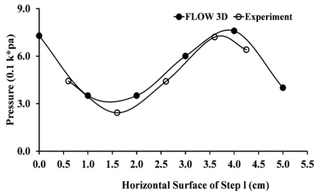
Fig. 3 FLOW 3D vs Experiment at horizontal surface
