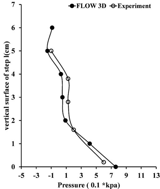
Fig. 2 FLOW 3D vs Experiment at vertical surface
