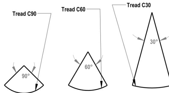
**Fig.05** Tread configurations for C30, C60 and C90
