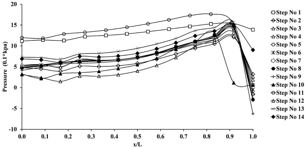
**Fig.9** Pressure profiles at horizontal surface of C90
