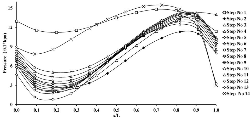
Fig.6 Pressure profile at the horizontal surface for C0 Step
