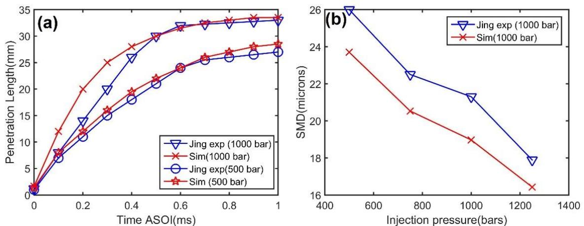
**Figure 4.** Comparison of simulated and experimental results [11] for a) PL and b) SMD respectively.
