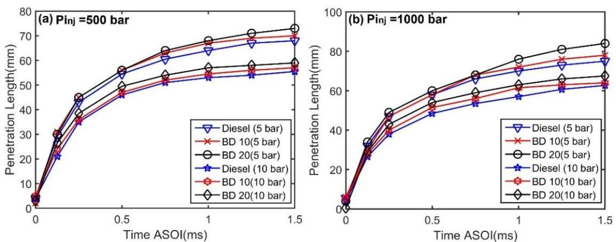
**Figure 5.** Penetration Length at Injection Pressure of a) 500 bar and b) 1000 bar respectively.
