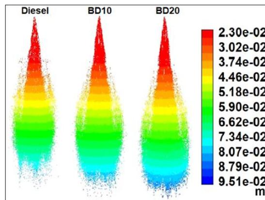
**Figure 6.** Penetration length contours at 1000 bar injection pressure.
