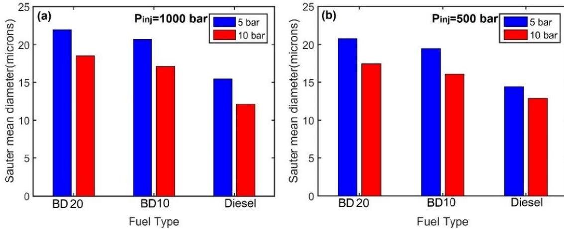
**Figure 7.** SMD for various fuels at a) 500 bar and b) 1000 bar injection pressure.
