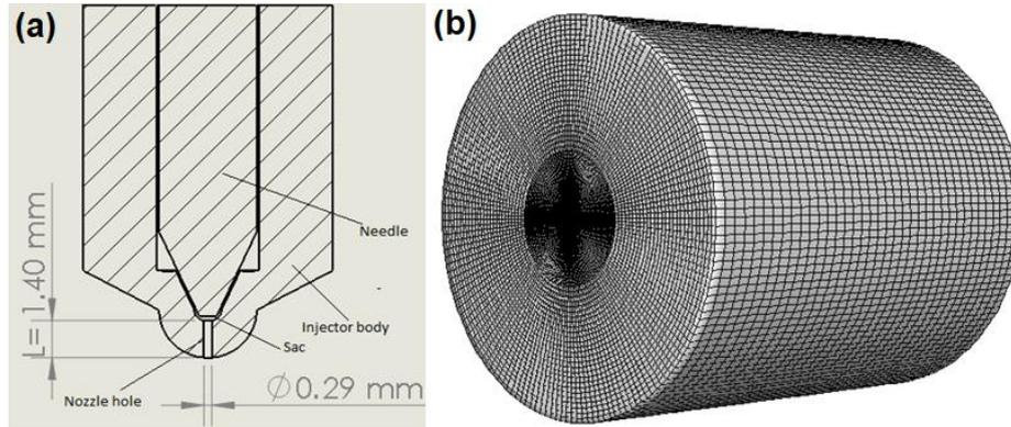
Figure 3. a) Injector nozzle, b) Computational domain
