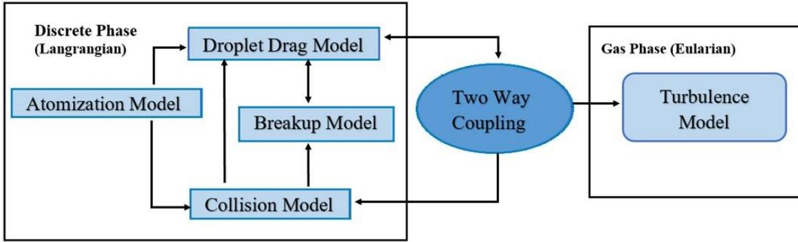
Figure 2. Numerical model interaction diagram for spray simulation.
