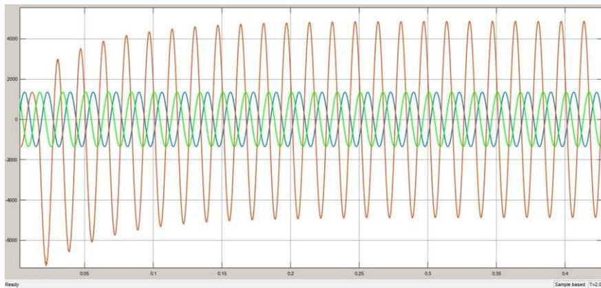
Figure 9 Sending Current when fault applied on Phase B
