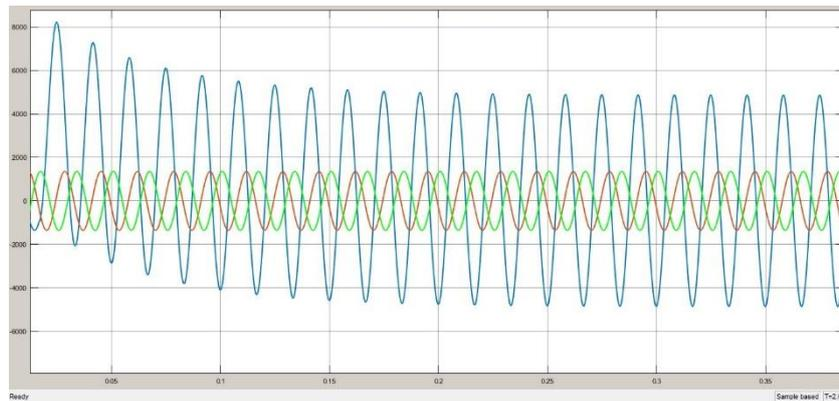
Figure 7 Sending Current when Fault applied on Phase A
