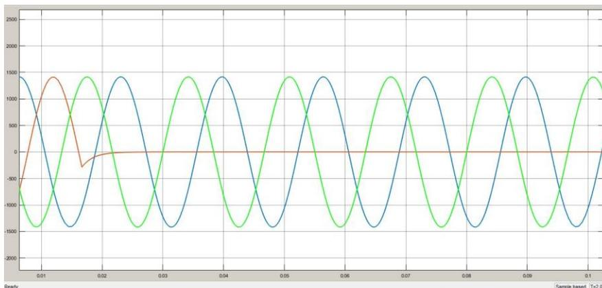
Figure 10. Receiving current when fault applied on Phase B
