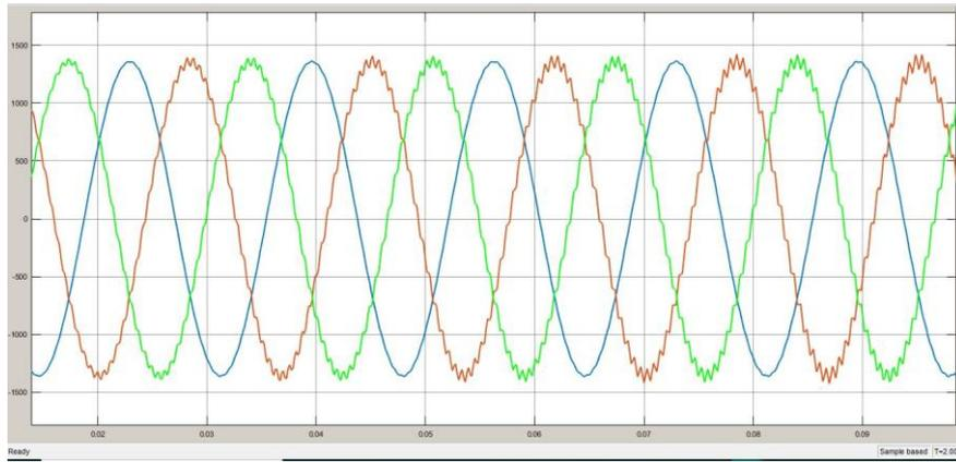
Figure 3 Sending Current before adding fault
