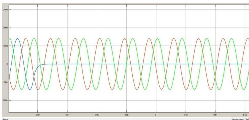
Figure 8 Receiving Current when fault applied on Phase A
