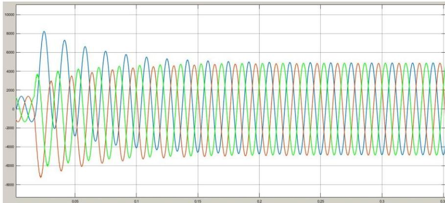
Figure 5 Sending Current after adding Three Phase Fault
