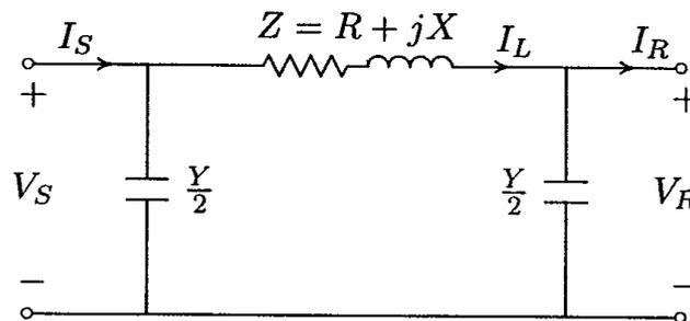
Figure 1. Nominal  $\pi$  model of for medium transmission line
