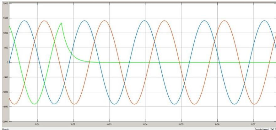
Figure 12 Receiving Current when fault applied on Phase C
