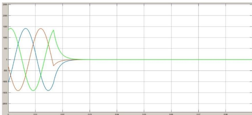
Figure 6 Receiving current after adding Three Phase Fault
