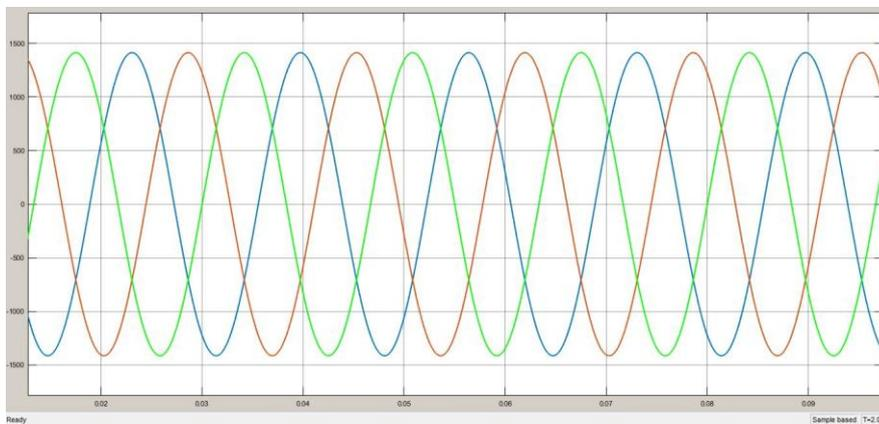
Figure 4 Receiving Current before adding fault
